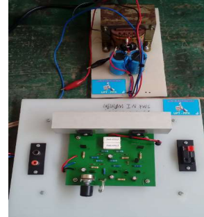
Gambar 12. Power Amplifier 75 W
