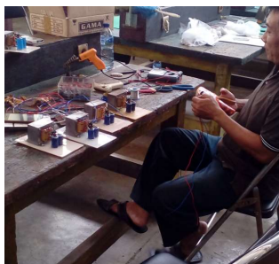
Gambar 11. Perakitan Power Supply
