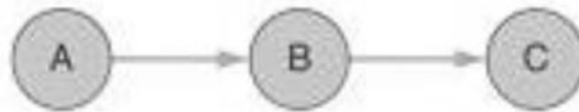
Figure 7. Activity A is the predecessor to Activity B, and Activity B is the predecessor to Activity C
