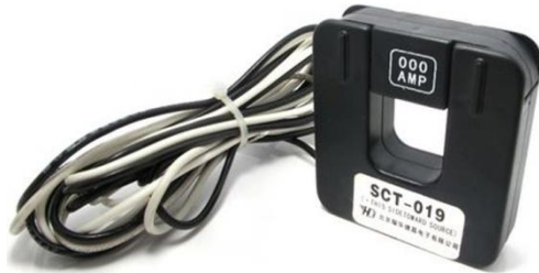
Gambar 8. Sensor Arus SCT 019
