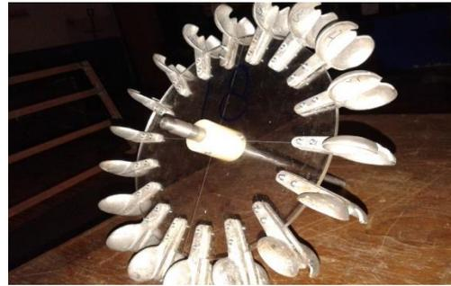
Gambar 13. Runner Turbin Air Pelton
