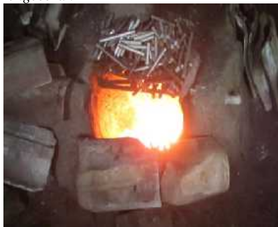
Gambar 2. Proses peleburan Al-6061
